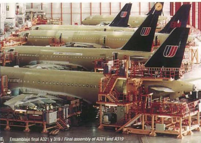
Ensamblaje final A321 y A319 / Final assembly of A321 and A319
