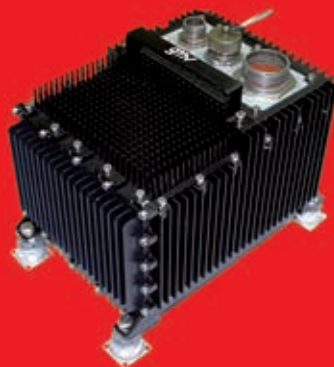
ATLANTE FCC (Flight Control Computer) responsible for the navigation, control and guidance of the aircraft.
